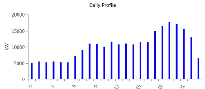
For the island of Martinique a HFO price of 21 US\$/GJ which is equal to about 0,78 €1 was set. A price increase towards 0,84 €1 is expected by 2028.[3]. The maximum PV size was limited to 20 MW given the space requirements of a PV plant, which allows for a maximum RES penetration of 50%. The maximum possible LCOE reduction is then about 18 % compared to an engine only system.
