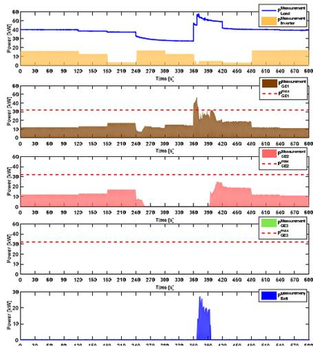
Figure 15 Power outage situation avoiding with storage integration
