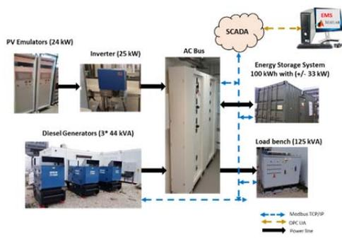
Figure 12 PV-Diesel hybrid system used for test
