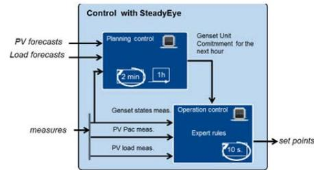
Figure 2 Two-levels control system
