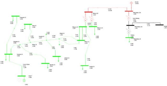
Figure 2: The 33 kV rural grid Mbeya to Tunduma
