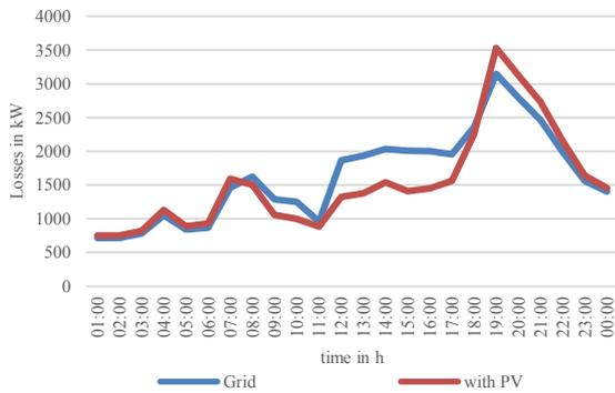
Figure 8: Grid Losses without control unit
