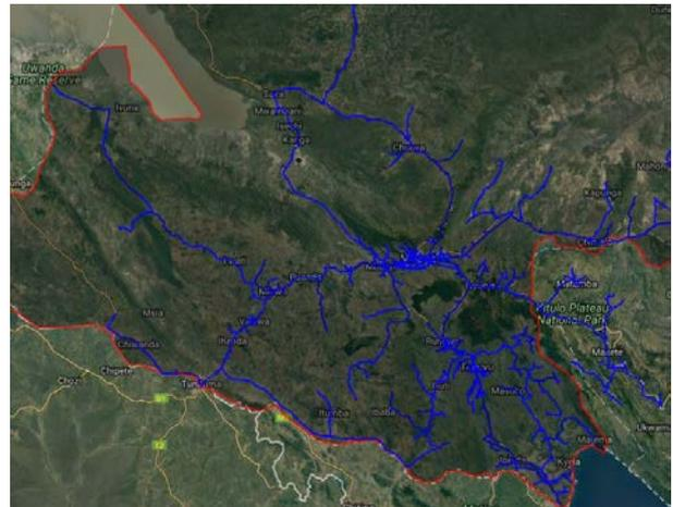
Figure 1: The 33 kV grid connected to Mbeya substation [1]
