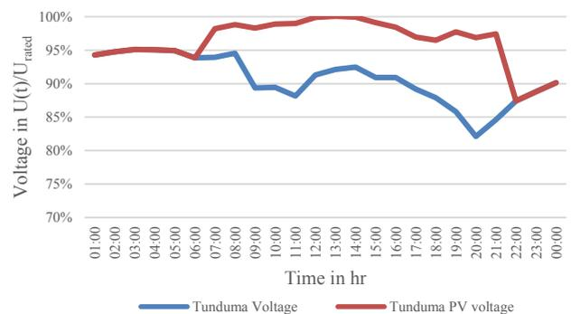
Figure 6: Voltage level Tunduma city
