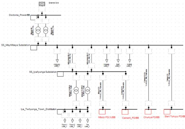
Figure 5: Power supply Mbeya and Iyunga substation
