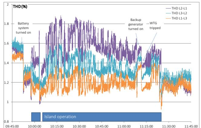
Figure 4– THD when islanded and grid connected 13<sup>th</sup> Dec 2017
