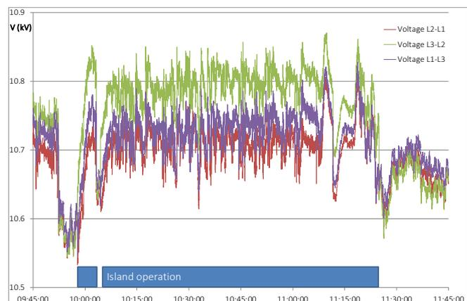
Figure 5 Voltage when islanded and grid connected 13<sup>th</sup> Dec 2017
