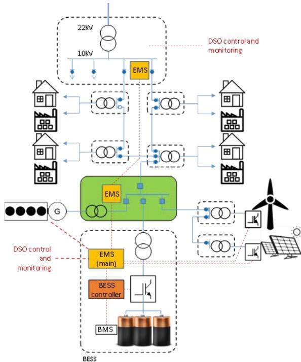
Figure 2 – Schematic over microgrid in Simris
