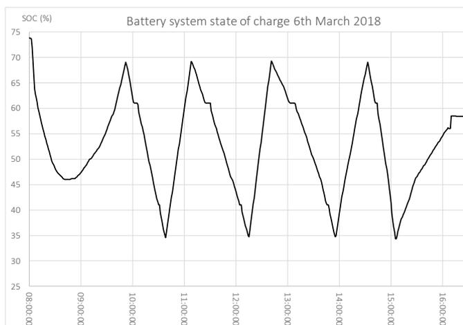
Figure 6 BESS SoC 6<sup>th</sup> March when the system was islanded 08:00 – 16:00
