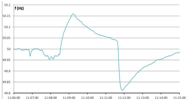
Figure 3 frequency from islanding test 13<sup>th</sup> December 2017
