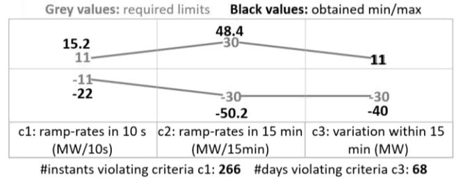
Figure 8. Expected fluctuations for the total PV power production along a year (with a ceiling of 11 MW in each 15 minutes)
