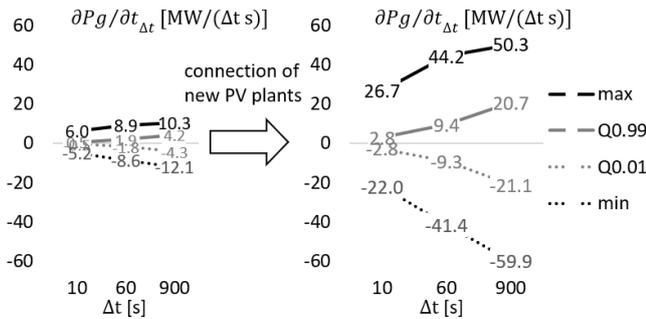
Figure 4. Expected ramp-rate values for the total PV power production along a year (statistical analysis)
