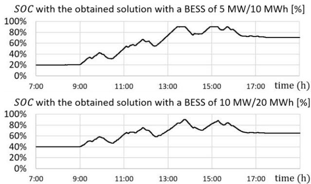
Figure 13. Expected SOC time evolution, in the illustrated disturbed day, if adopting one of the feasible control solutions
