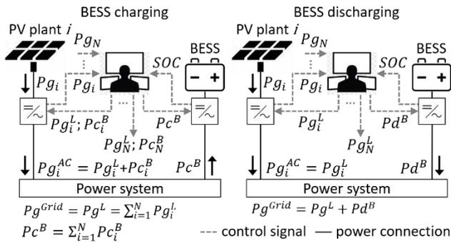
Figure 6. High-level architecture of the control system
