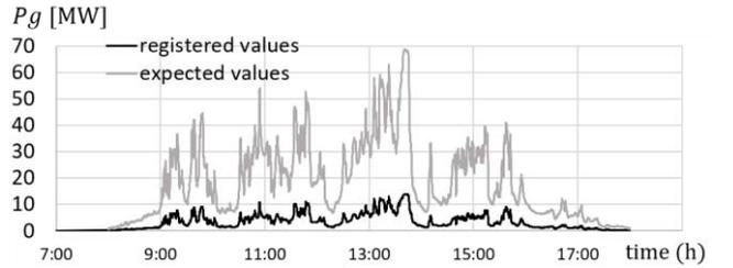
Figure 1. Daily time series of the total PV power production in a disturbed day (registered and expected values)
