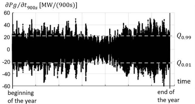
Figure 5. Annual time series of the 15-min ramp-rates for the expected total PV power production
