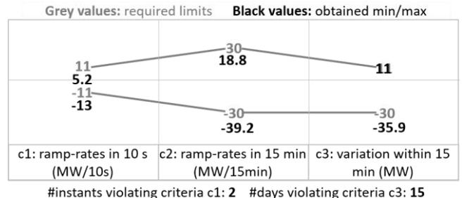
Figure 9. Expected results (ceiling: 11 MW; max ramp-up: 1%/min applied in new PV plants)
