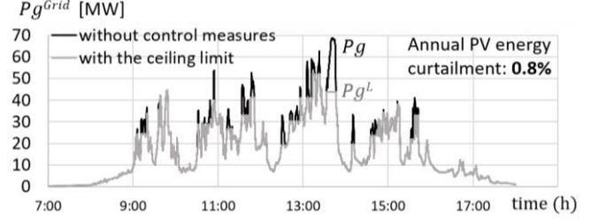
Figure 7. Expected total PV power production in the illustrated disturbed day (with/without ceiling limit = 11 MW in each 15 minutes)
