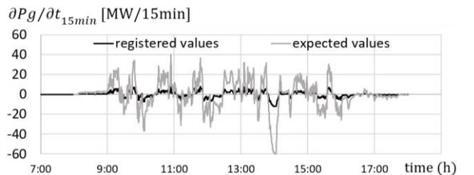
Figure 2. Daily time series of the 15-min ramp-rates for the total PV power in a disturbed day (registered and expected values)
