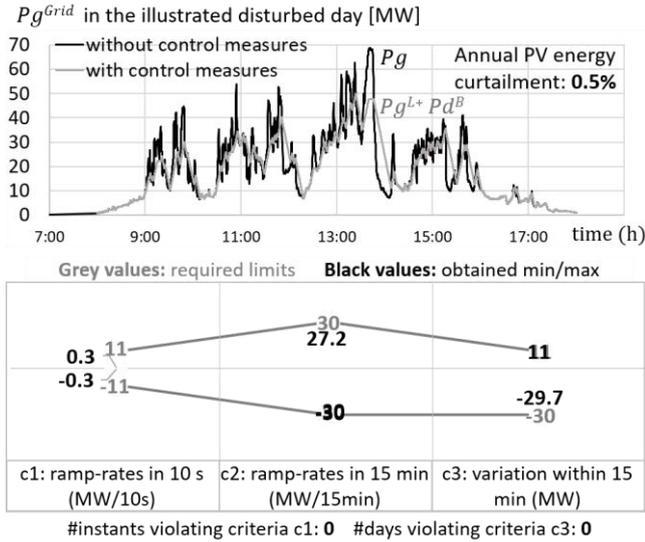
Figure 12. Expected results with a BESS of 40 MW/30 MWh without MPPT control (ceiling: 11 MW; ramp-rate limits  $\pm 2.7\%/min$  applied in all PV plants)
