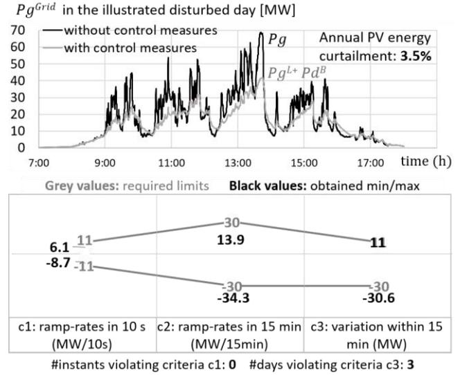
Figure 10. Expected results with a BESS of 5 MW/10 MWh (ceiling: 11 MW; ramp-rate limits  $\pm 0.5\%/min$  applied in new PV plants)
