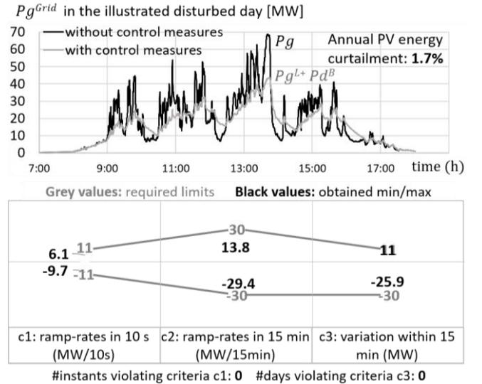
Figure 11. Expected results with a BESS of 10 MW/20 MWh (ceiling: 11 MW; ramp-rate limits  $\pm 0.5\%/min$  applied in new PV plants)
