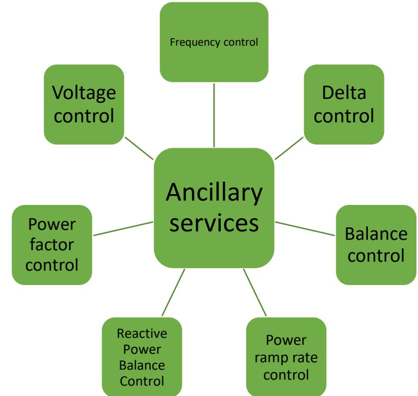
Figure 6. Basic ancillary services provided by power system generation
