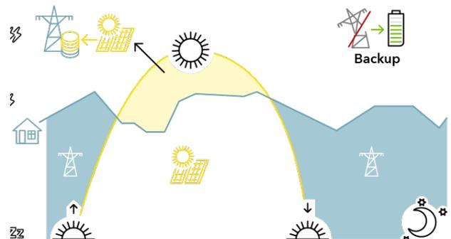
Figure 4: Grid connected installation with full grid feeding: the battery is not cycled (kept for backup only):
