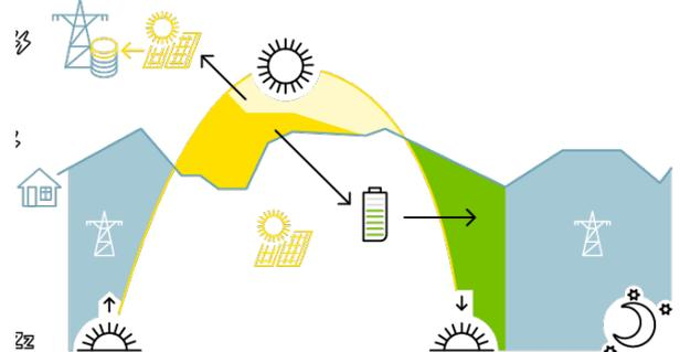
Figure 3: Grid connected installation with grid feeding allowed and use of battery for self-consumption optimization:
