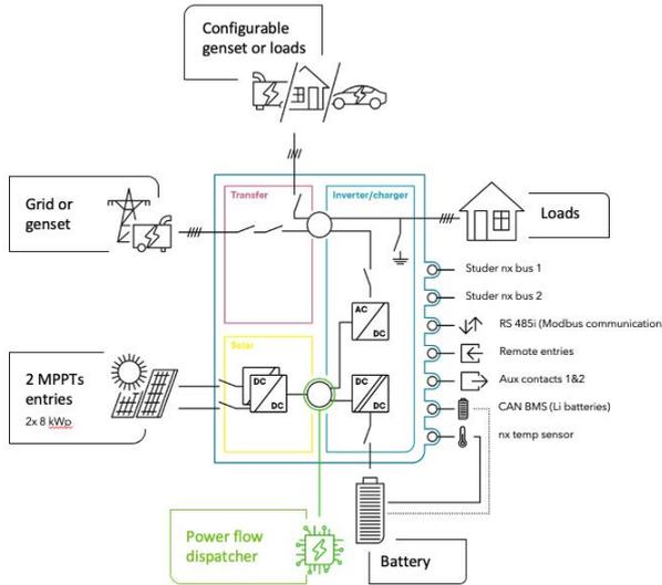
Figure 1: Internal architecture of the hybrid power inverter
