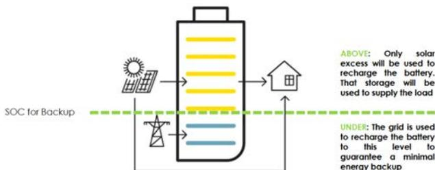
Figure 7: Principal usage of the battery storage
