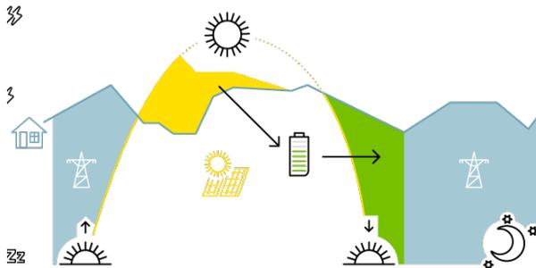
Figure 5: Solar priority without grid feeding: zero export solar backup
