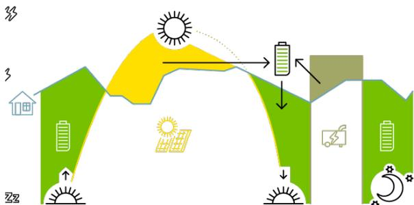
Figure 6: Off-Grid installation (back feeding on genset is forbidden!)
