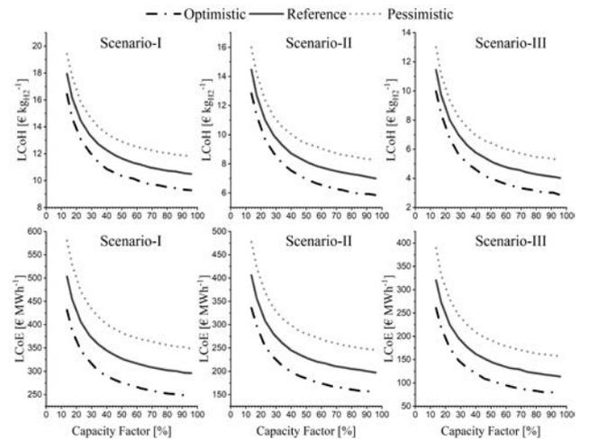
Figure 3 Variation of LCoE (PtP conversion) and LCOH (net fuel production cost) for the selected scenarios across all annual equivalent full load hour operations [9].
