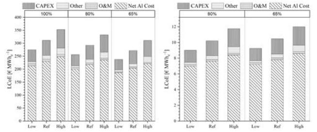
Figure 2 LCoE and LCoH estimations for the base case, i.e., 4000 FLHs and electricity price of 50 €MWh<sup>-1</sup> under varying operation modes (100%, 80%, and 65% SOFC partial load (Low: lower end, Ref: reference, and High: higher end.) [9].
