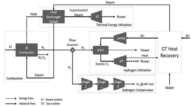
Figure 1. Simplified Al wet combustion plant layout showing main energy and material streams [9].
