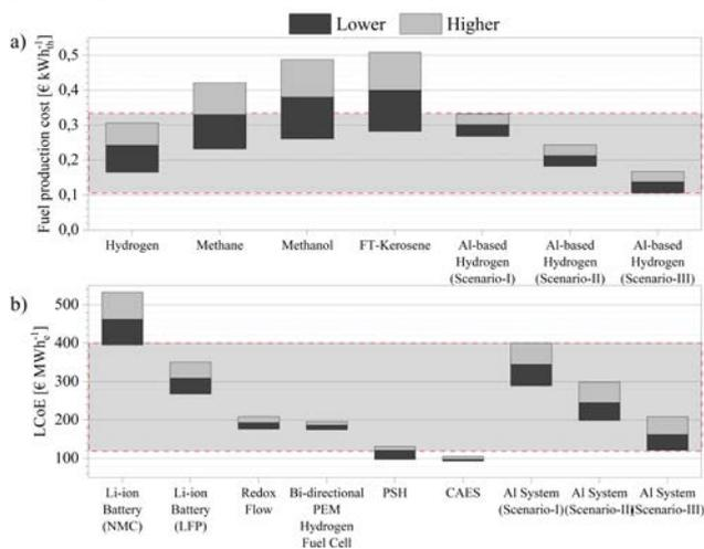
Figure 4 a) Comparison of net fuel production costs based on 4000 FLHs, and b) LCoE of various storage technologies based on power-to-power conversion path. (The power capacity of the selected technologies for comparison is 100 MWe and estimated LCoE values are based on the assumed 10 h of daily storage duration.) FT Kerosene: Fischer-Tropsch-synthesis kerosene, NMC: nickel-manganese-cobalt, LFP: lithium-iron-phosphate, PSH: pumped storage hydropower, CAES; compressed air energy storage.) [9].
