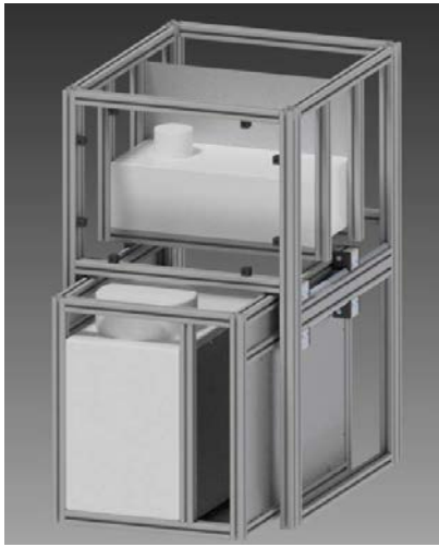
Figure 3: Basic disinfection setup with feed tank (below) and FAC tank (on top).
