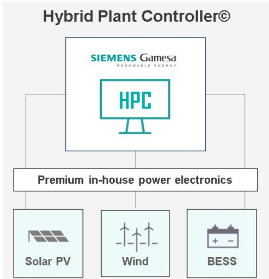
The HPC is the brain of the Hybrid plant it controls all the assets within a Hybrid Plant to ensure, grid connection compliance, revenue and asset longevity maximization.
