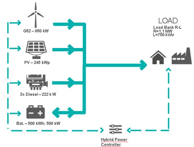
The HPC “Hybrid Power Controller” manages, in real time, the mix of the 4 energy sources: Wind, Solar PV, Storage (2 different technologies) and Diesel. Load is either provided by the grid or simulated using an Active and Reactive Power Load Bank by which a wide variety of load scenarios can be tested.
