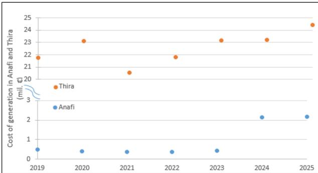
Figure 7: Total generation cost over the Interconnection study horizon, for the ESs of Anafi and Thira.
