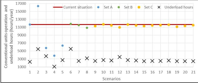
Figure 3: Number of operation hours of conventional units for each scenario for the Hosting Capacity Study for the NIIPS of Anafi.
