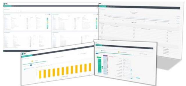
Figure 1: Screenshots from the Application. Upper left: Dashboard. Upper right: Demand/Peak model. Down left: RES (PVs) capacity. Down right: conventional units parameters fields.
