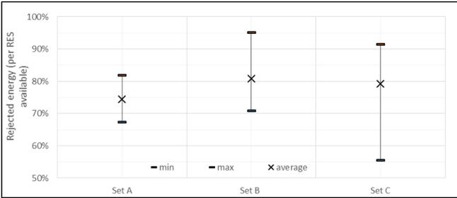
Figure 4: Range of rejected RES energy (per RES available) per scenarios set for the Hosting Capacity Study for the NIIPS of Anafi.
