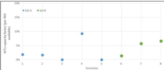
Figure 5: WT's capacity factor (per RES available) for Set A and B for the Hosting Capacity Study for the NIIPS of Anafi.
