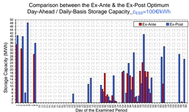
Figure 8. Optimized, daily-basis ex-ante and ex-post storage capacity.
