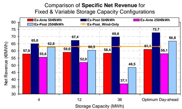
Figure 12. Specific net revenue for different storage configurations.
