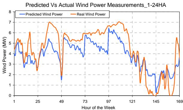
Figure 4. Actual vs day-ahead predictions of wind power generation.
