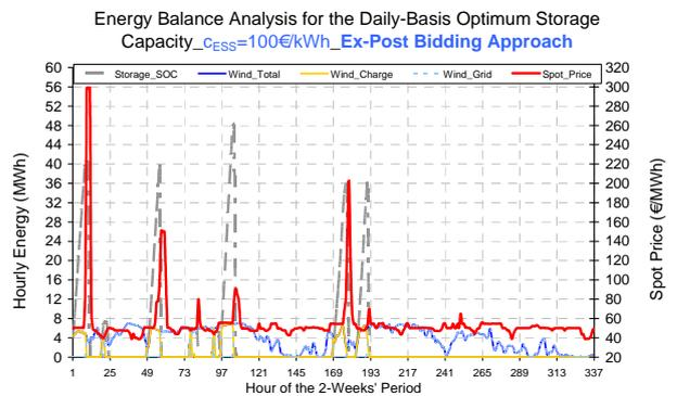
Figure 7. Ex-post, optimum daily-basis wind-storage bidding profile.
