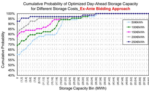
Figure 9. Optimum, ex-ante storage capacity probability curves.
