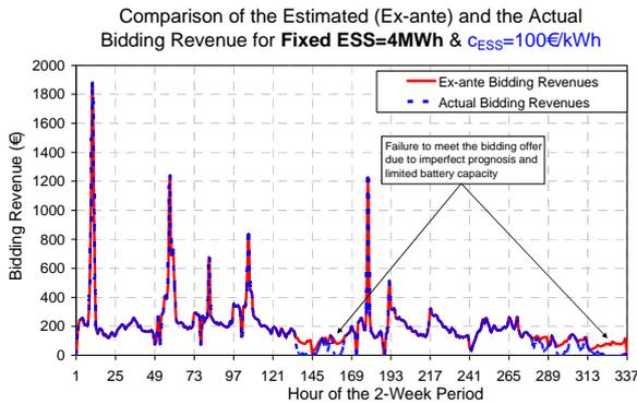
Figure 14. Design vs actual revenue for fixed storage capacity of 4MWh.
