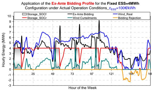
Figure 13. Design vs actual operation for fixed storage capacity of 4MWh.
