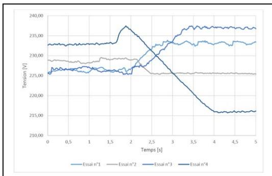
Figure 8 ESS RMS voltage during several islandings
