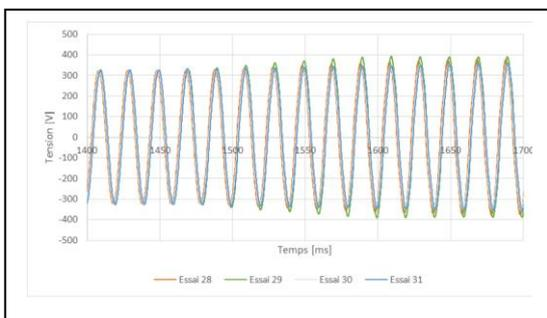
Figure 9 Voltage wave form during several islandings
