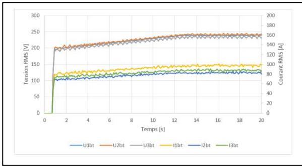
Figure 7 Voltage and current during a blackstart
