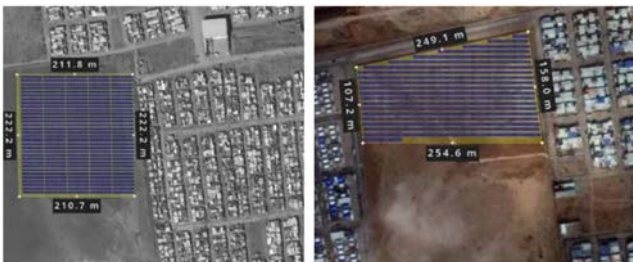
Figure 3: 6.6 MW solar PV installation in Domiz 1 (left) and a 2.5 MW solar PV installation in Domiz 2 (right)
