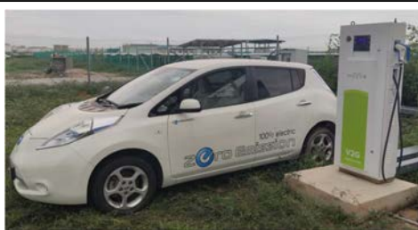
Figure 5 Electric Vehicle with V2G charging station
