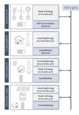
Figure 3. Different type of users in the mini-grid
