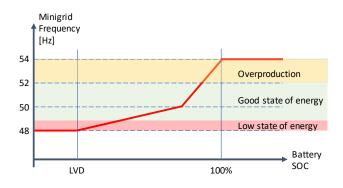
Figure 4. Frequency behaviour of the central inverter according to the battery voltage
