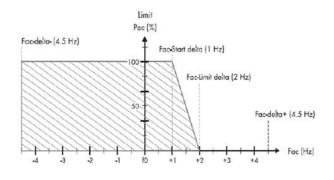
Figure 8. Frequency shift control for AC-coupling grid-tied inverters
