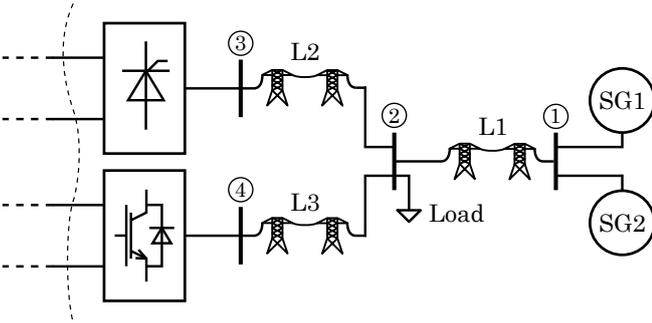
Fig. 2: Case study of multi-infeed islaned system with an LCC and a VSC-HVDC links
