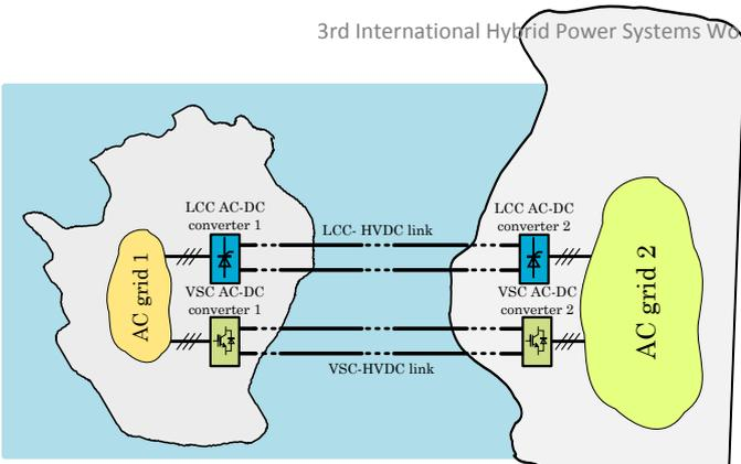
Fig. 1: Example of multi-infeed HVDC islaned system
