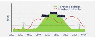
As volatile generation grows, integration becomes difficult. To avoid its curtailing (switching it off), two alternatives exist: Energy storage
